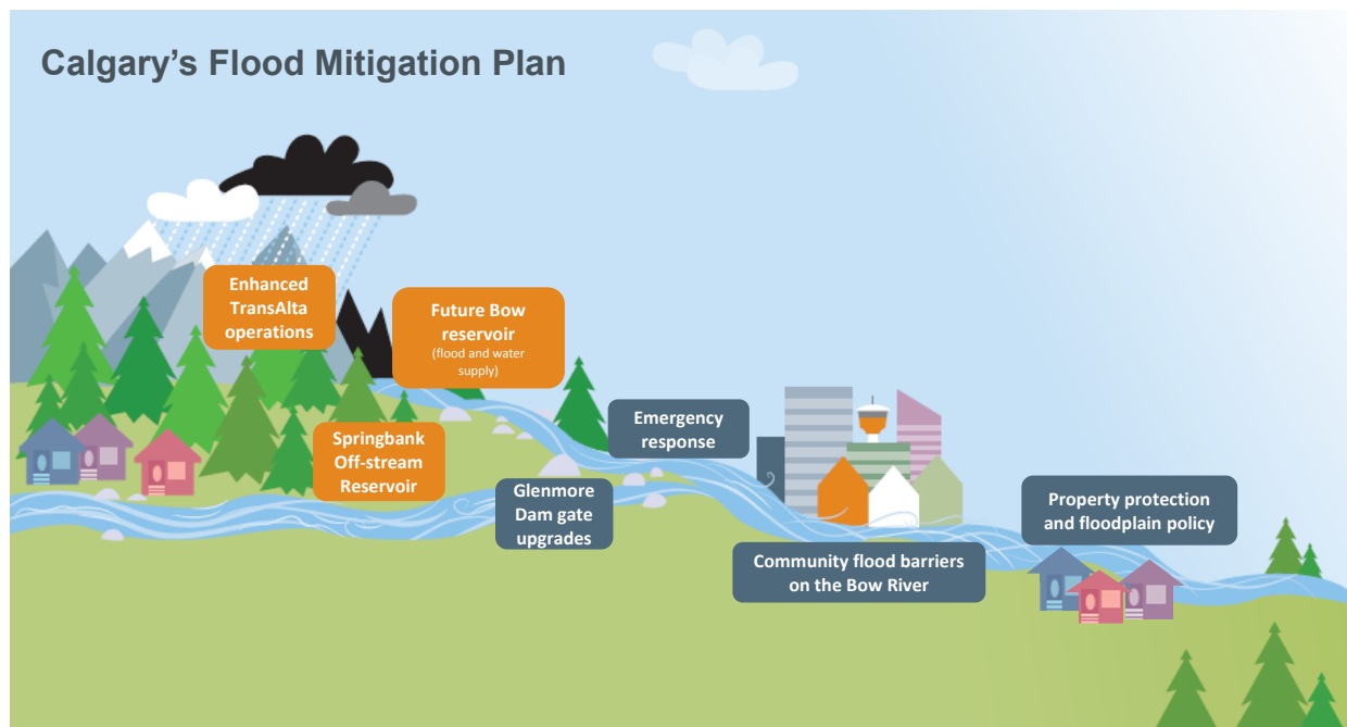
FIGURE 1 CALGARY'S PLAN RELIES ON UPSTREAM AND COMMUNITY INVESTMENTS, OPERATIONS, PROPERTY PROTECTION AND FLOODPLAIN POLICY
